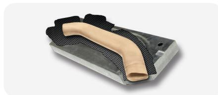
**2 • Drape forming:** Carbon fabric layers (prepare) are placed around the bladder, inside the aluminium female mould.
