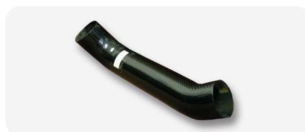
**4 • Removal from the mould:** once the curing is complete, the bladder is deflated and the mould is opened; the bladder removed and the part is sent for finishing.
