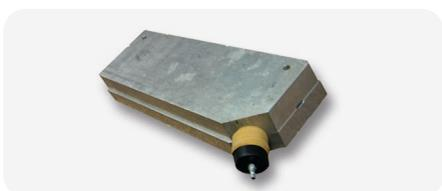
**3 • Curing:** after the mold is closed, the bladder is inflated to plate the prep-reg in the mold (up to 6 or 8 bars), then we proceed to the curing.
