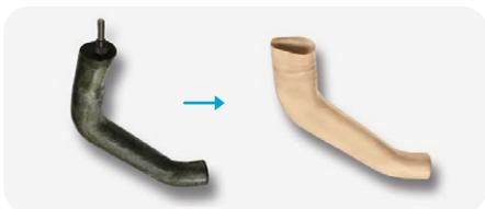
**1 • Dipping:** to the left, the aluminium male mandrel and to the right, high temperature natural rubber bladder manufactured by dipping.
