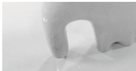
The mold is dipped in a coagulant bath then in a high temperature natural latex bath. The thickness of the layer depends on the dipping time. After vulcanization, the bladder is removed from the dip mold.
